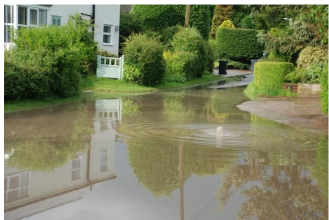
Low point in Peppin Lane (note surcharged sewer cover discharging) during Storm Babet Oct 23
